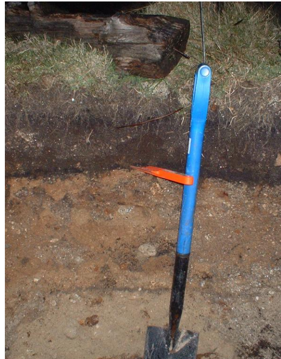
21 THE SOIL PROFILE with organic soil above the orange trowel and mineral soil below.
