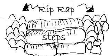
91 RipRap used at steps to stop walking or cycling to the side of the step which can lead to water damage.
